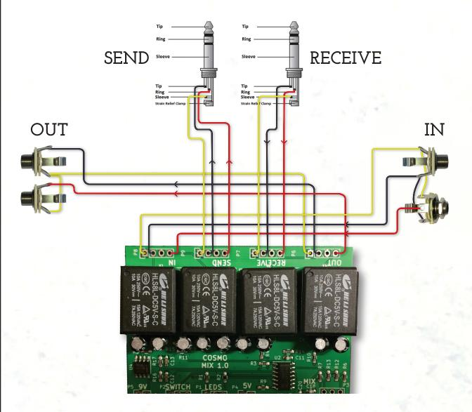
If you're using a RCA cable instead of 3,5mm Jack for the send/receive, then ground should be connected to both left and right cable, while center conductor of the left and right cable should be connected to the left and right connections on the send and receive respectively.
